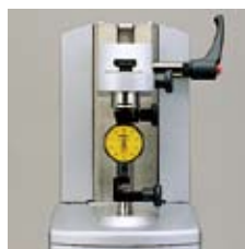
Using test indicator attachment set (02ASK000)
